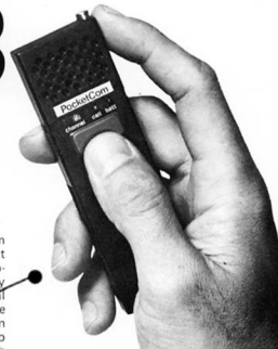
The PocketCom measures approximately 3/4" x 1 1/2" x 5/8" and easily fits into your shirt pocket. The unit can be used as a personal communications link for business or pleasure.
